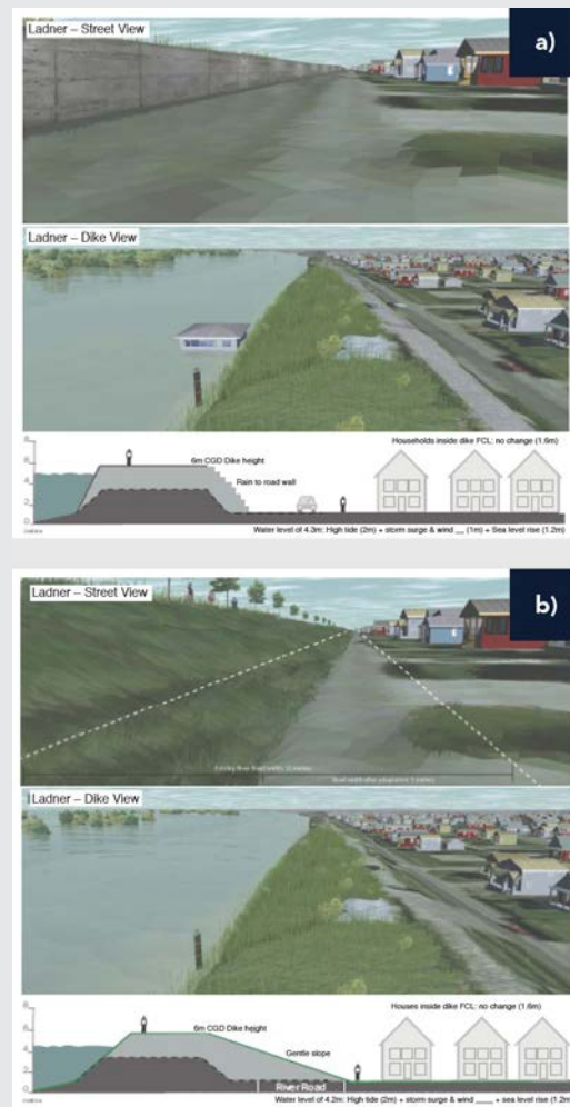
FIGURE 14: Visual models of potential adaptation options. Images are of Ladner (part of the Corporation of Delta) with a larger dike and berm in 2100 with 1.2 m of sea-level rise. The dike has been built up accordingly, and the images show two design options: a) a steep concrete-reinforced wall that would maintain the current right-of-way for River Road; and b) a conventional design that would take up half of one of the main roads. Source: Corporation of Delta. Created by Collaborative for Advanced Landscape Planning (CALP), University of British Columbia.
