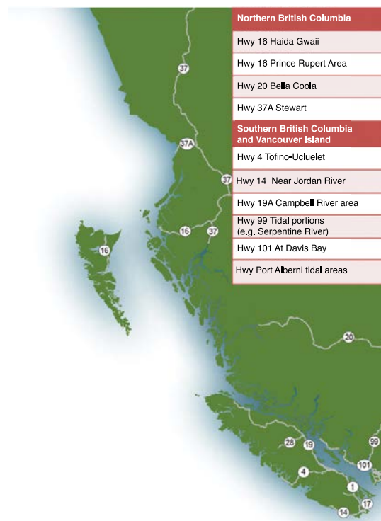
FIGURE 22: Areas of provincial coastal highways identified as being at risk from sea-level rise (modified from D. Nyland).
