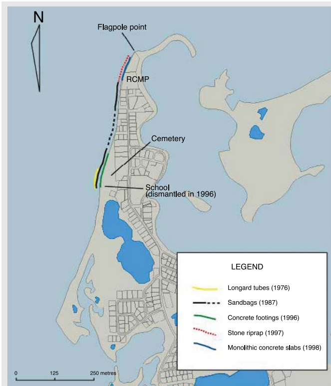
FIGURE 22: Location of various shore protection measures installed at Tukttoyaktuk to help control erosion and flooding (from Couture et al., 2002).
