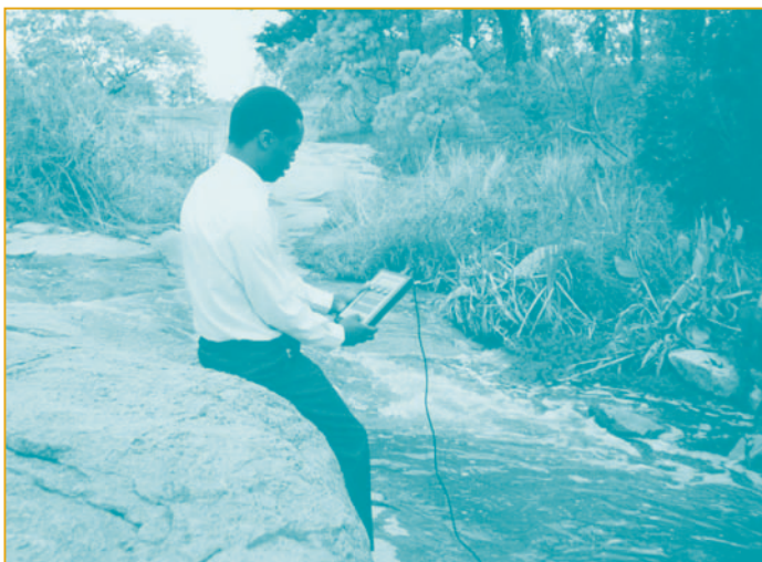
Figure 37. Flow measurement using an integrating meter (photo courtesy of Dulas Engineering Ltd.)
