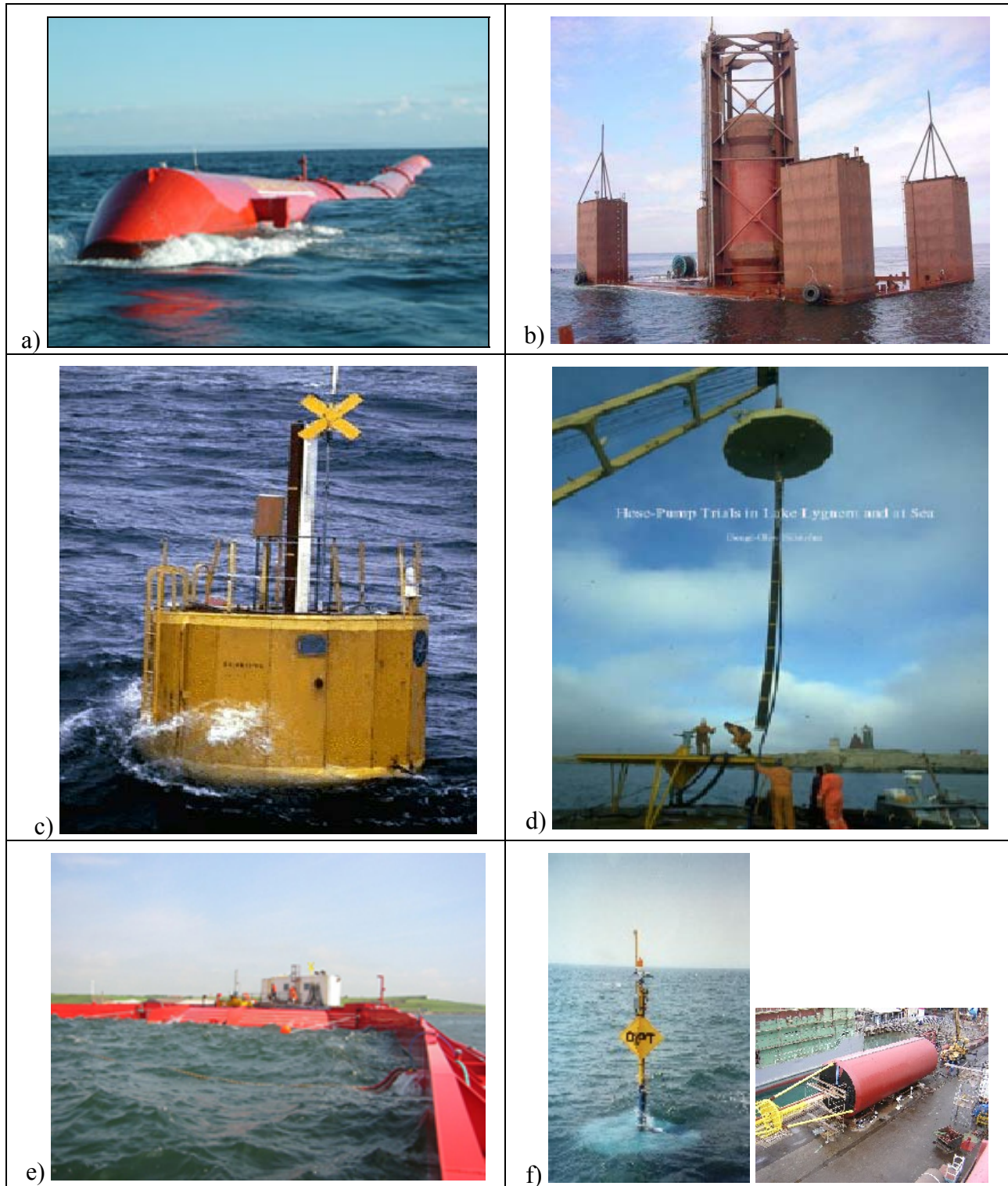
Figure 4. Six examples of offshore wave energy converters: a) Pelamis; b) Archimedes Wave Swing; c) IPS Buoy; d) Technocean Hose-Pump; e) Wave Dragon; f) OPT PowerBuoy.
