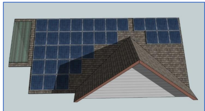
Figure 17: Example of Self-Induced Array Shading by Roof Gable - courtesy of Riverside Energy Systems
