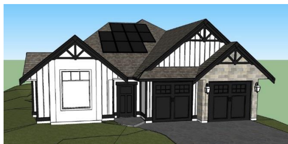
Figure 4: South Dormer Removed in Favour of 3 kWp PV Array – courtesy of Sonbuilt Homes
