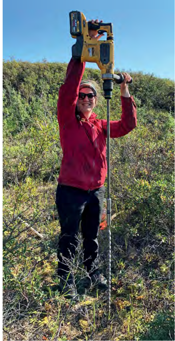
Drilling a borehole for a thermistor in a revegetated thaw slump in the Beaufort Delta region of the Northwest Territories
