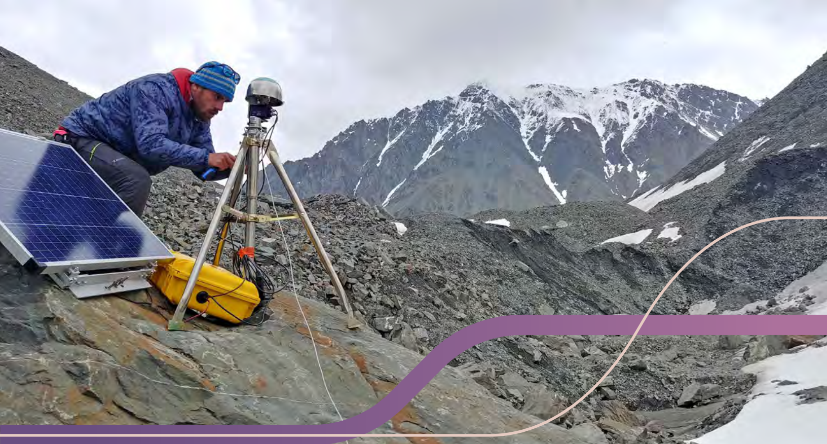
Installing an autonomous LiDAR station to monitor topographical changes in a buried ice area
