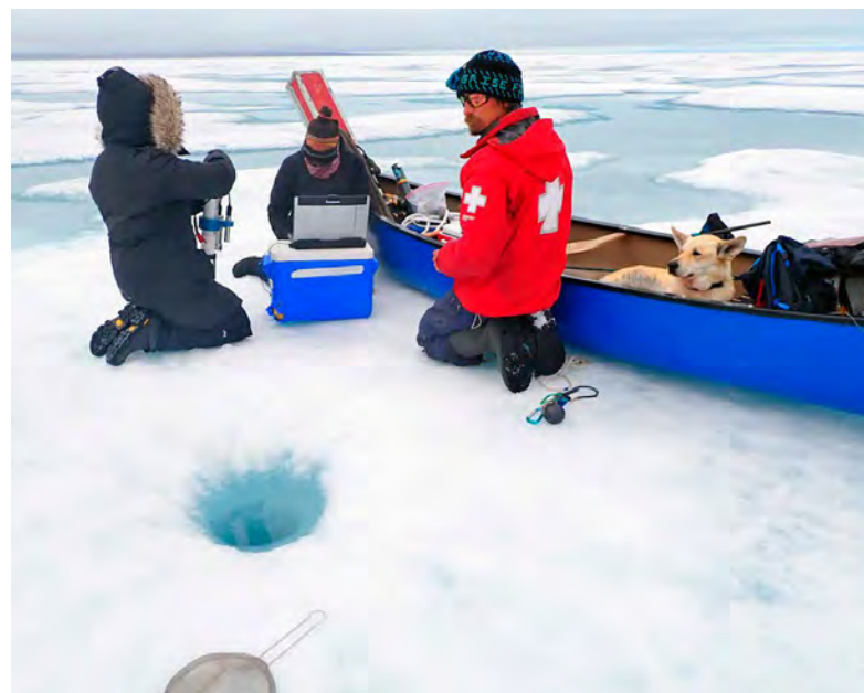
The team deploys a conductivity, temperature and depth instrument to measure the salinity, temperature and other characteristics of seawater.
