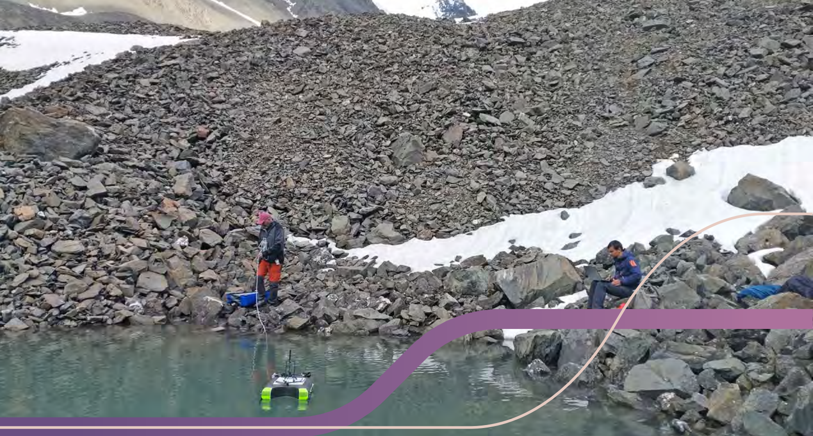
Surveying the bathymetry of a temporary lake on a rock glacier with an acoustic Doppler current profiler
