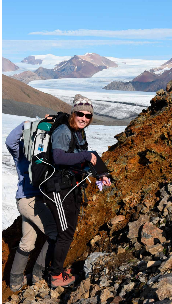
Measuring the spectral signature of the iron hats to improve its reference data for classifying the geology of the region
