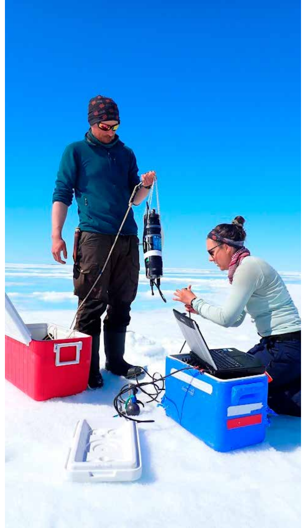
Deploying instruments to measure CO 2 dissolved in seawater
