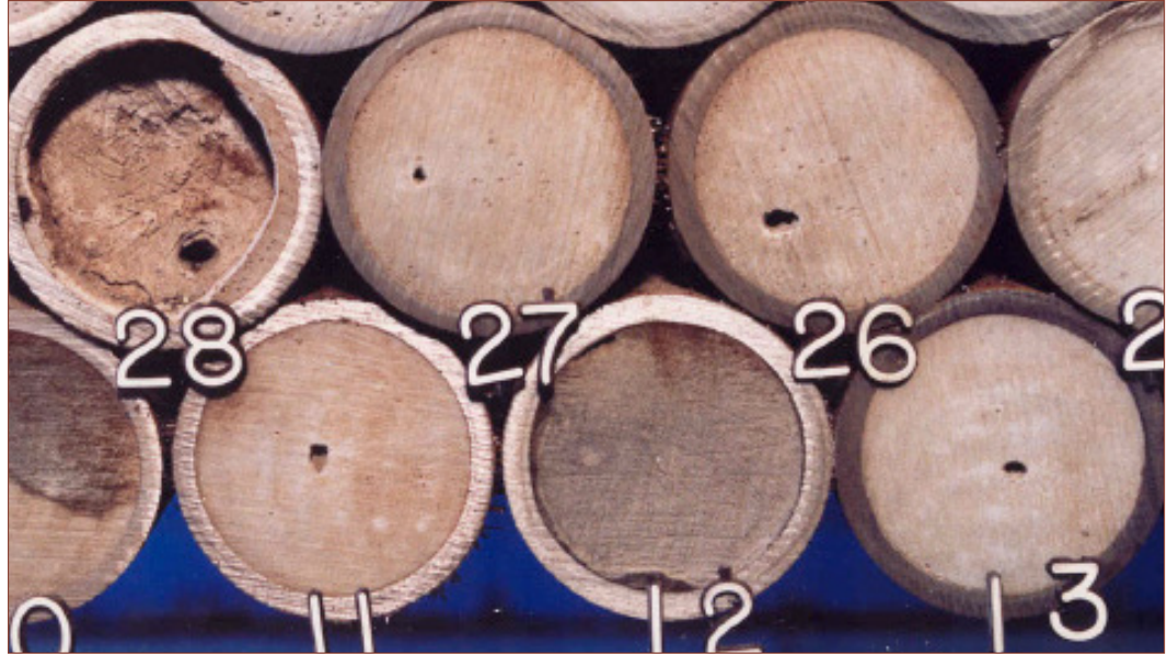
Figure 4.3 Gas channels and gas pockets formed in set cement as a result of gas migration (Watson et al., 2002).
