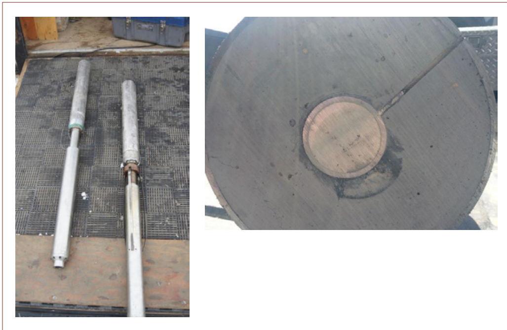
Figure 6.1 Seal Well alloy deployment tools with bismuth-tin alloy cast on the outside of a cartridge heater. The technology can be used to both seal wells for abandonment and remediate leaky wells. In either application, the tool is lowered onto a mechanical bridge plug and the heater is turned on. The second image is of a wellbore analogue system with an alloy-filled perforation (Spencer and Lightbown, 2015).
