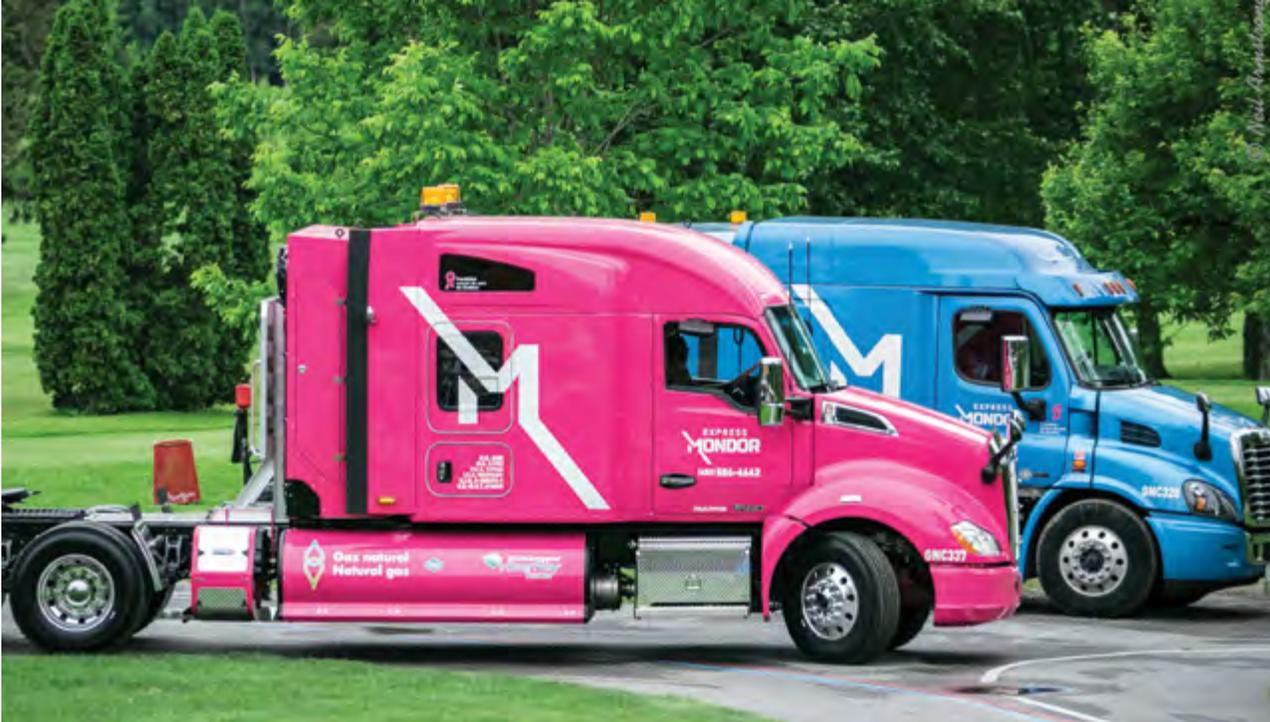
Kenworth T680, Cummins engine ISX12N, Eaton autoshift transmission, Agility tank with 210 DGE capacity, painted for the Quebec Breast Cancer Foundation
