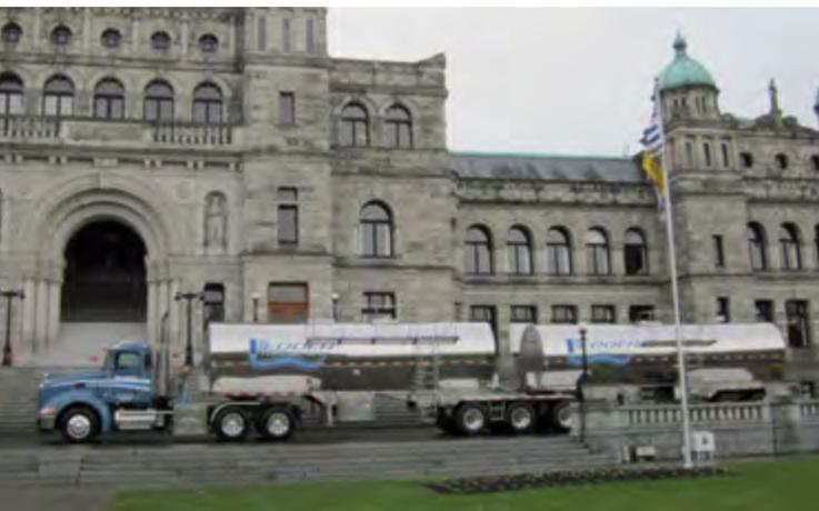
Vedder B-Train at the British Columbia Legislature in Victoria, B.C., Peterbilt 386 with a high pressure, direct injection, LNG-modified, Cummins engine
