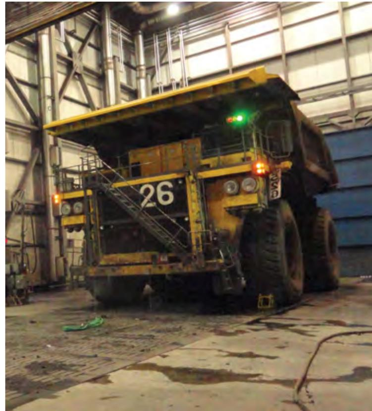
Ore-hauling vehicle in service at a Canadian coal mine enters a maintenance facility equipped to service natural gas vehicles
