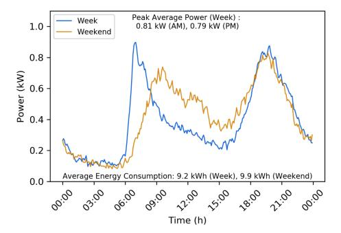
Figure 11 – 24-Hour Electrical Profile – Spring
