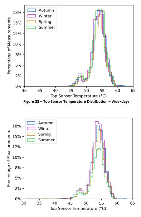
Figure 24 – Top Sensor Temperature Distribution – Weekends
