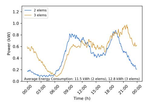
Figure 13 – 60 imp gal 2 elements vs 3 Elements Winter Electrical Profile – Weekends
