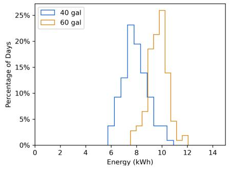
Figure 19 – Average Daily Energy Consumption Distribution – 40 imp gal vs 60 imp gal
