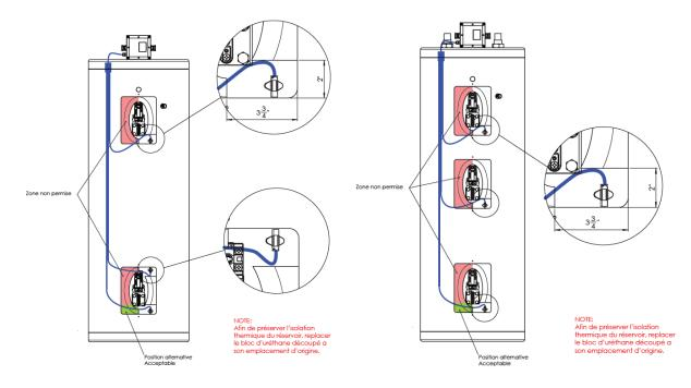
Figure 6 – Location of Temperature Sensors in Two-Element (Left) and Three-Element (Right) EWHs
