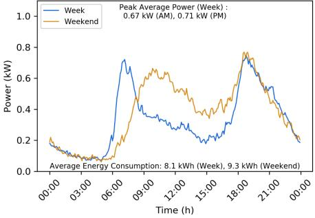
Figure 10 – 24-Hour Electrical Profile – Fall
