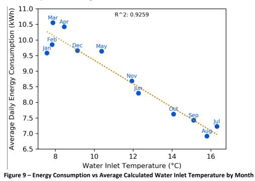
It is noted that the calculated water inlet temperature is negatively correlated to the average daily energy consumption ( $R^2 = 0.926$ ). These results are once again coherent:
