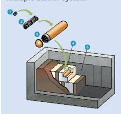
Within a deep geological repository, a series of engineered and natural barriers will work together to contain and isolate used nuclear fuel from people and the environment. Each of these barriers provide a unique and stand-alone level of protection. If any of the barriers deteriorate, the next one comes into play. For more information on the multiple-barrier system that the NWMO is using to safely contain and isolate used nuclear fuel, please visit www.nwmo.ca/multiplebarriersystem.
