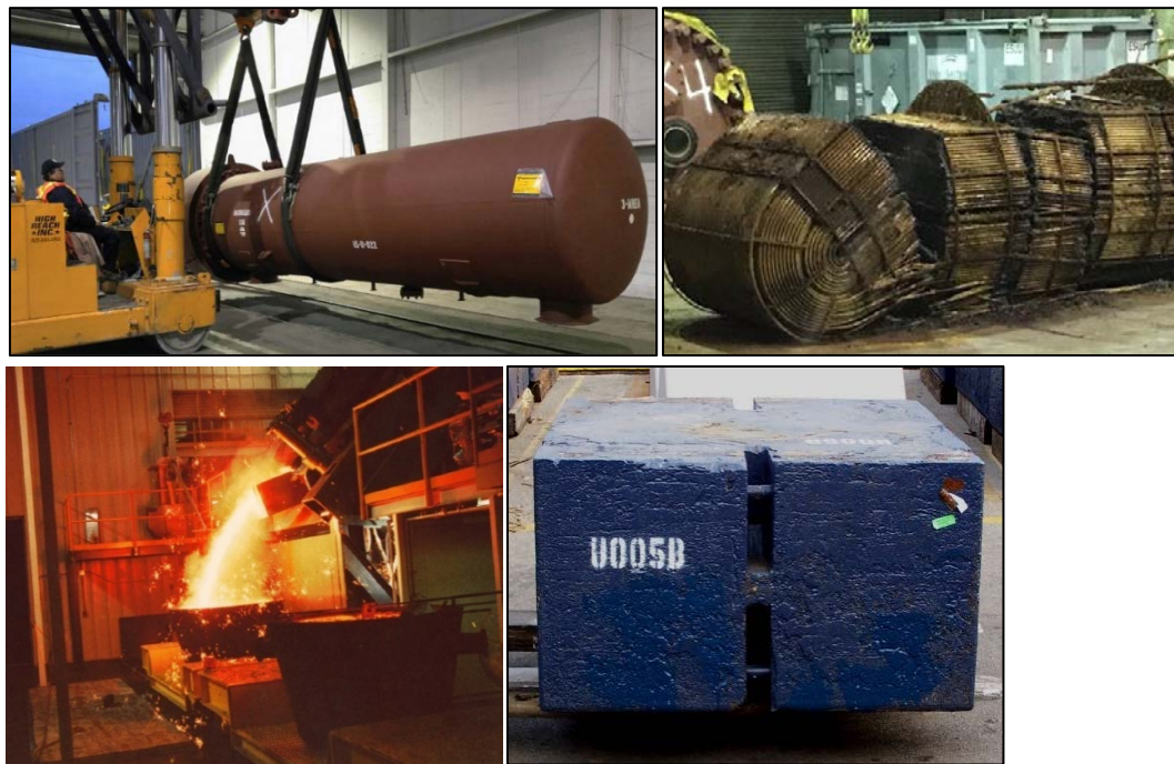
Figure 6: A heat exchanger first is segmented, then processed via metal melting. The resulting metal ingot is then re-used within the nuclear industry as a shielding block
