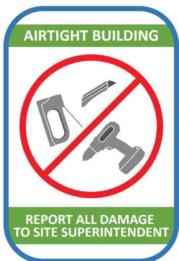
Figure 33 Example airtightness sign to use on site for notifying all staff and trades
