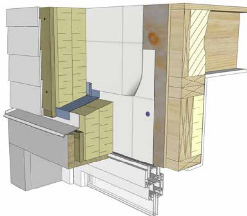
Figure 21 Window head flashing with through-wall flashing membrane lapped beneath the field membrane.
