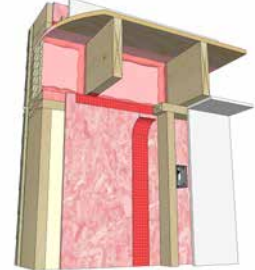
Sealed Interior Sheathing
