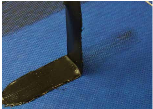
Figure 3 Sealant adhesion test showing adhesive failure from a synthetic vapour-permeable self-adhered membrane.
