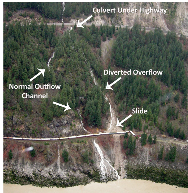
Figure 14: Komo, British Columbia train derailment caused by debris flow onto train tracks. (Source: Transportation Safety Board of Canada)
