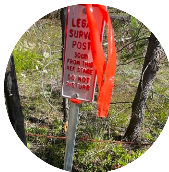
Example of a metal reference post
