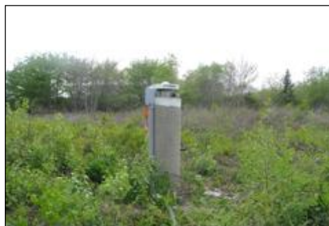
Figure 4 : Ground based, concrete pillar monument
