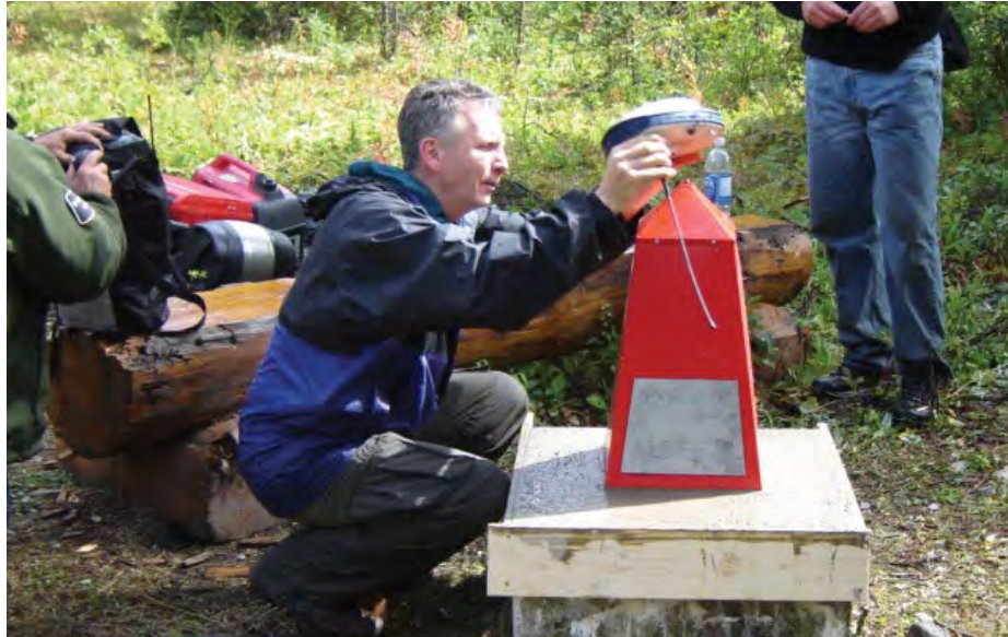
Figure 5. SGB's Jim Mackenzie taking GPS measurements on monument 1N of the Alberta–British Columbia boundary.
