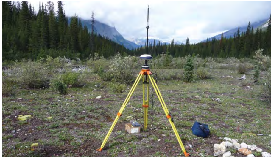
Figure 2. Precise Point Positioning (PPP) and Real Time Kinematic (RTK) GPS for legal surveys — Banff National Park.
