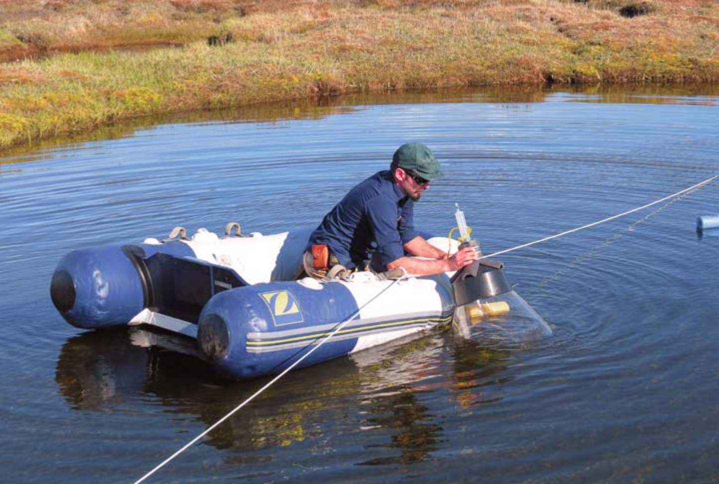
Installing an inverted funnel in a polygonal pond of the Qarlikturvik Valley in Sirmilik Park, Bylot Island, to measure the methane that is released from the pond sediments and contributes to the greenhouse effect
