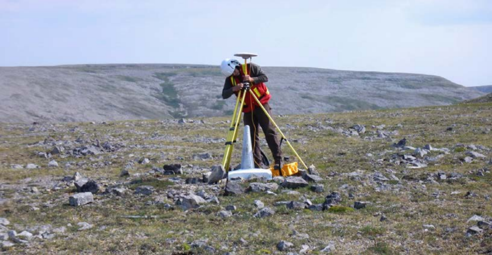
Setting up a GPS receiver on a boundary marker that marks the Yukon-Alaska border while surveying along the 141st meridian
