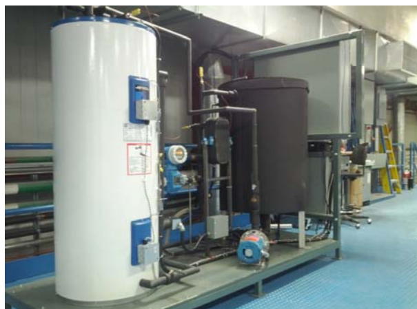
Figure 2: Demand Response test bench with an electric water heater
