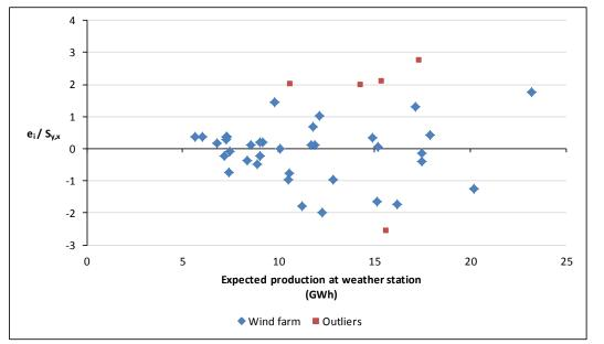
Figure 16. Standard error from regression analysis of monthly production data for a sample wind farm.
