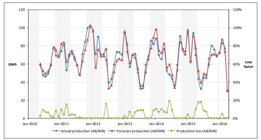
Figure 17. Monthly actual and forecast energy production in GWh (left axis) and production loss as percentage (right axis), aggregated for wind farms in Alberta and Manitoba.
