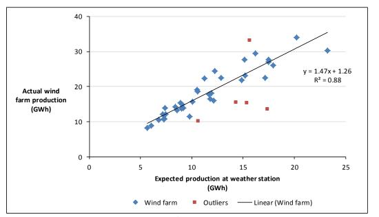
Figure 15. Actual production (from WPPI/EcoERP) vs. expected production at weather station for a sample wind farm, monthly data.
