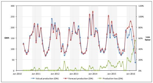
Figure 18. Monthly actual and forecast energy production in GWh (left axis) and production loss as percentage (right axis), aggregated for wind farms in Ontario.
