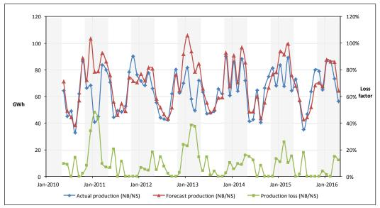
Figure 20. Monthly actual and forecast energy production in GWh (left axis) and production loss as percentage (right axis), aggregated for wind farms in New Brunswick and Nova Scotia.
