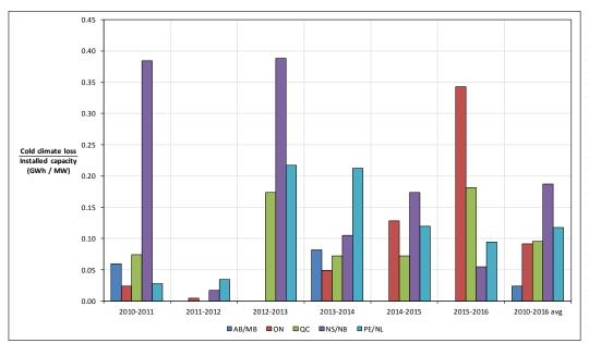
Figure 12. Cold climate energy losses, normalized by the installed wind energy capacity for each region in the study group.
