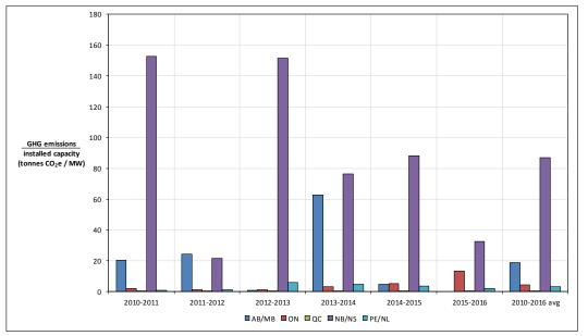
Figure 13. GHG emissions resulting from cold climate losses, normalized by the installed capacity for a given region and year.
