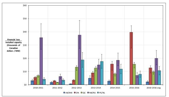
Figure 14. Financial losses resulting from cold climate losses, normalized by the installed capacity for a given region and year.
