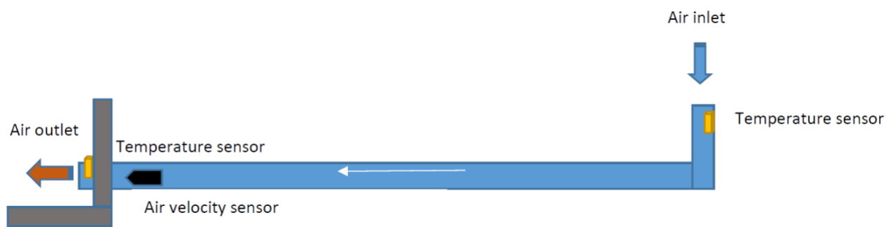
Figure 20: Location of Temperature and Air Velocity Sensors
