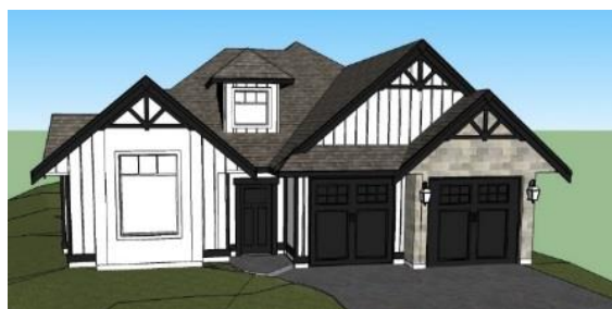
Figure 3: South Roof Dormer Limits South Facing Solar PV – courtesy of Sonbuilt Homes
