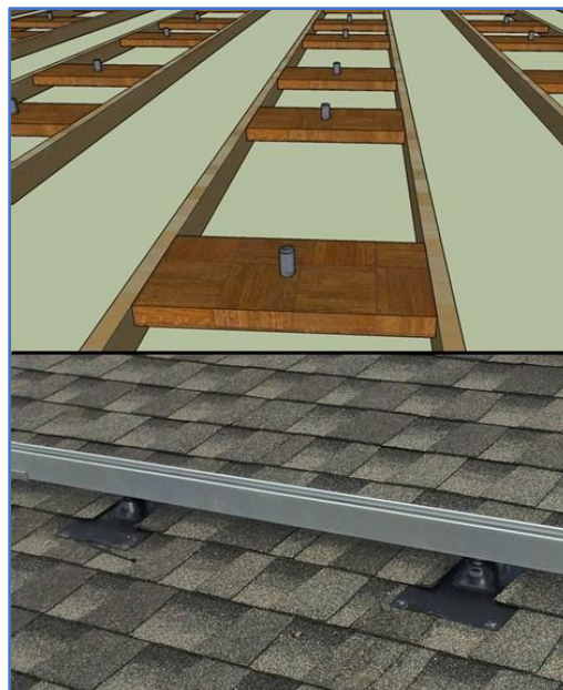
Figure 24: Lag Bolted Anchors to Blocking between Trusses: - Sub-structure (top); Flashed Anchors with Racking (bottom) - courtesy Riverside Energy Systems
