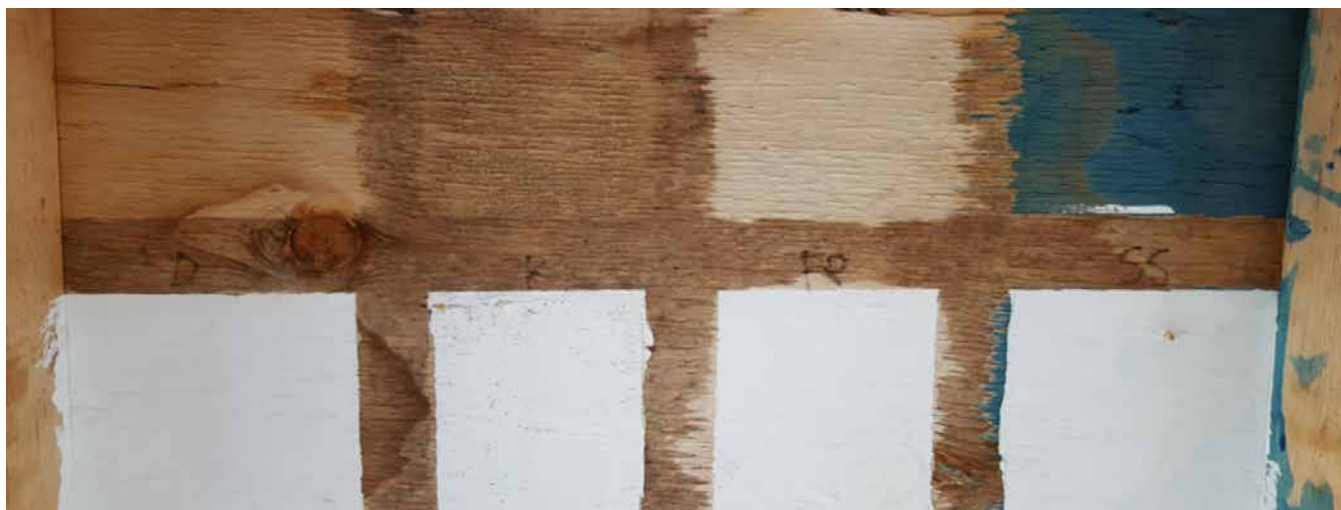
Figure 4 Test panel showing different coating treatments applied to clean wood to compare their effectiveness in limiting microbial growth.
