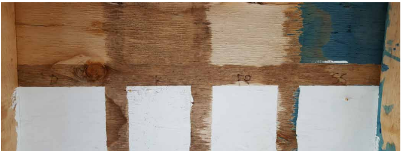
Figure 7 Test panel showing different coating treatments applied to clean wood to compare their effectiveness in limiting microbial growth.
