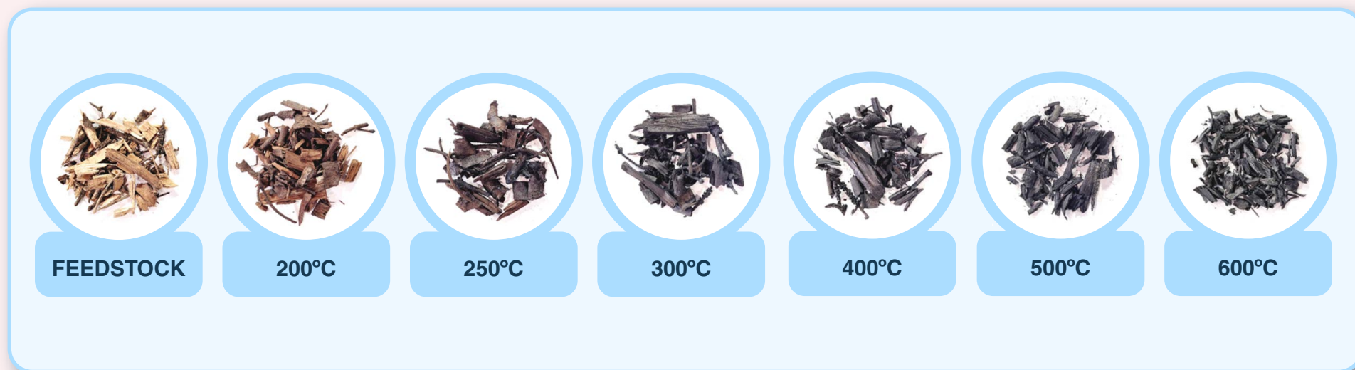
Figure 1: Visual progression of forest residues through pyrolysis at increasing temperatures (200°C to 600°C)
